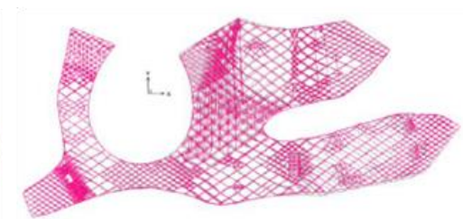
Mode 7 ( f_7=1.417 Hz) Translational vibration along X axis.
