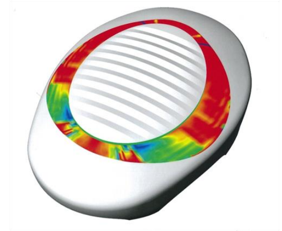
Gaussian curvature analysis ( -2.65e-12 \sim 2.65e-11 )
