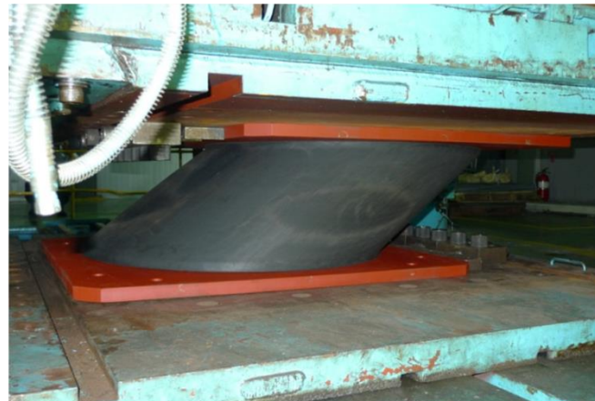
<LRB8000 Maximum displacement pre-test>
